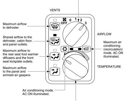
Rotating the selector simultaneously opens and closes the hot and fresh air butterfly valves, permitting conditioned (mixed) air to enter distribution system.
