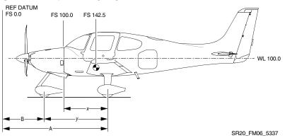
Basic empty weight, moment, and center of gravity are provided in inches aft of datum, where 0 inches datum is 100.0 inches forward of the cabin firewall. CG can also be expressed in terms of its location as a percentage of the airplane Mean Aerodynamic Cord (MAC) using the following formula:
