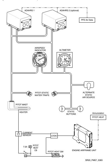
Figure 7-16: Pitot-Static System - Serials w/ MD302 (2 of 2)
