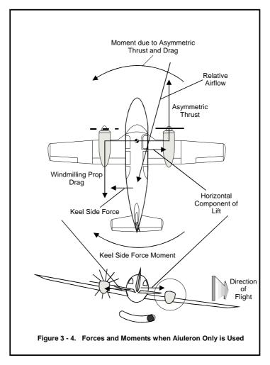
Provided sufficient bank is used, the horizontal component of lift will be equal to the fuselage side force, and the aircraft will now maintain a straight flight path without any rudder applied, but with a significant amount of slip towards the operating engine. Again, this slip will cause an increase in form drag. In this condition the balance ball will be well displaced towards the operating engine.
