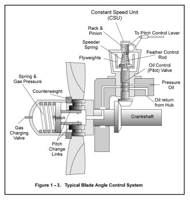
However, a possible problem arises in the event of a mechanical engine failure in flight which causes a rapid reduction in RPM. If this occurs, and the propeller control lever is not moved to the "feather" position before the centrifugal latches engage, the propeller blades will not feather.
