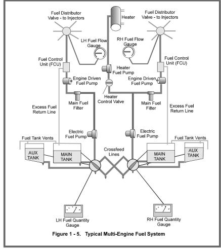
A typical twin-engine fuel system is shown in Figure 1 - 5
