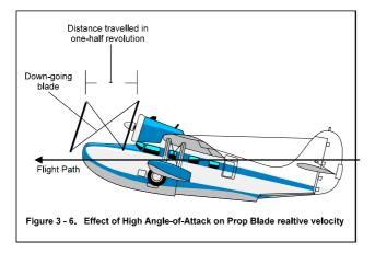
However, when an engine fails the loss of thrust and increase in drag will cause the aircraft to decelerate, requiring an increased angle of attack to maintain level flight. At high angles of attack, the propeller discs are no longer at right angles to the flight path, ie, the relative airflow.
