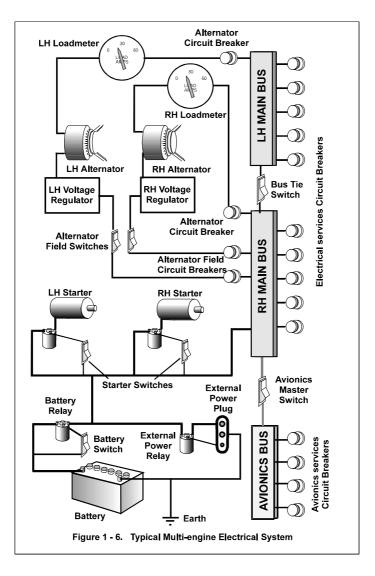
Although some of the older twins are still fitted with generators, the remainder of this Section will refer only to alternators. Figure 1 - 6 is a schematic diagram of a typical light twin electrical system.
