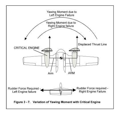
To overcome the problem of a "critical engine" some manufacturers install counter-rotating engines so that the down-going propeller blades are closest to the centre of gravity. This minimises the yawing moment caused by asymmetric thrust at high angles of attack, and also means that neither engine is "critical".
